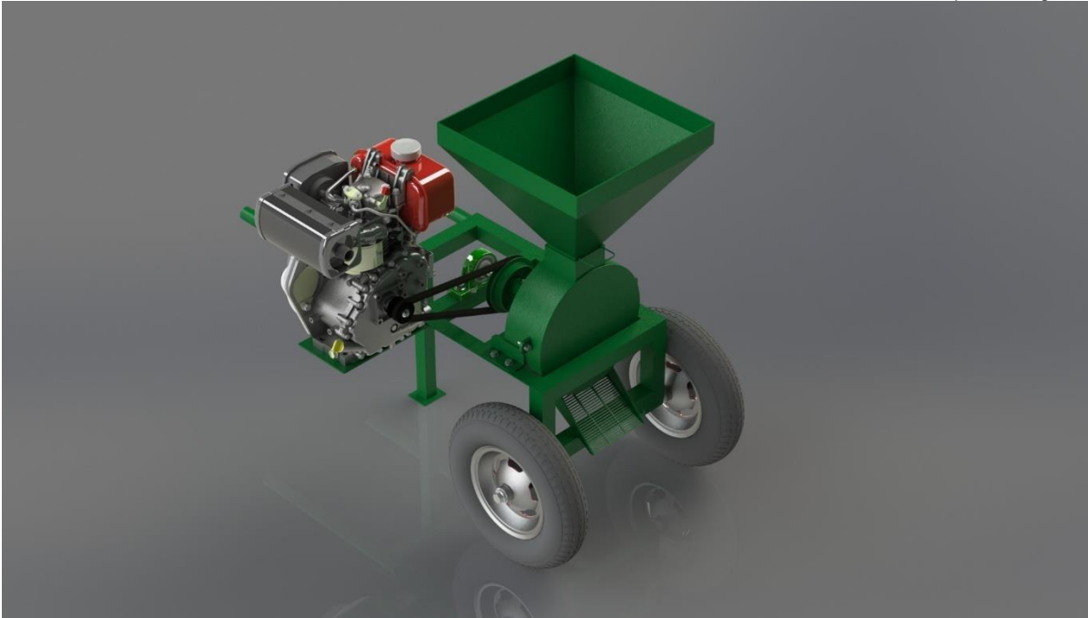
Figure 2.1: Three dimensional model of the developed palm kernel nut cracking machine
